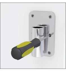
**Step 5: Tighten Screws equally.** Tighten each screw in an alternating sequence pattern until bracket is firmly pressed to the wall without movement. This will limit risk of cracking wall surface.
